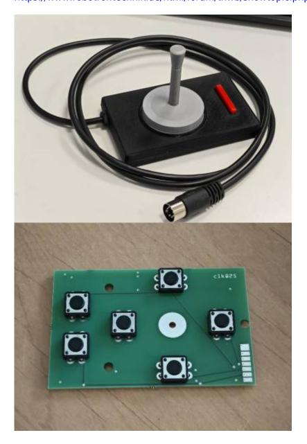
Taster: 12 x 12 x 4.3 mm Plate Mini/Micro/Small PCB Push Button
