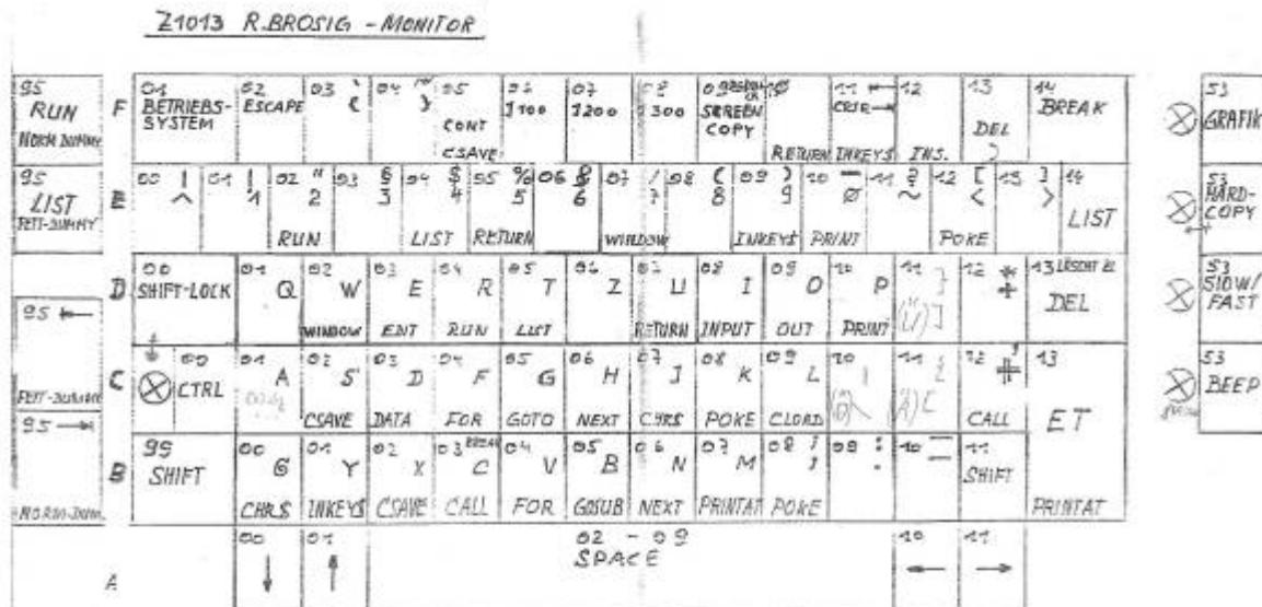
W=WINDOW E=EDIT R=RUN F=LIST U=RETURN I=INPUT O=OUT P=PRINT C=CSAVE D=DATA F=FOR H=NEXT G=GOTO L=LOAD
